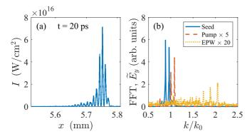
FIG. 4. PIC simulation of a DFBRA as in Fig. 3 but with an initial phase difference of  $\pi$ . The spectra (b) of the amplified seed (solid blue), pump (dashed red), and EPW (dotted yellow) is similar to that without initial phase difference (Fig. 3) but the intensity of the amplified pulse (a) has a maximum at the center of the beat-wave envelope.
