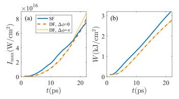
FIG. 5. A comparison between the dynamics of SFBRA (solid blue) and of DFBRA with initial relative phase differences of zero (dashed red) and  $\pi$  (dotted yellow). Presented are the maximum intensities (a) and total fluences (b) versus the propagation time of the amplified pulse in the plasma.
