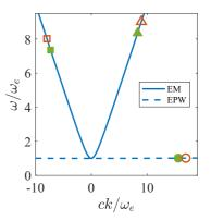
FIG. 1. Illustration of the doubly three-wave interaction in  $(\omega - k)$  space. The frequencies and wave numbers of the pumps (triangles), the seeds (squares), and the EPW obey the resonance conditions of Eqs. (8) and (11) for both indices 1 (filled points) and 2 (empty points). The solid and dashed lines are the dispersion curves of the EM wave and the EPW, respectively.
